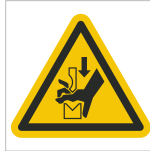
Hand crushing between press brake tool
