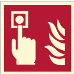
Fire alarm call point
