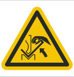
Hand crushing between press and material
