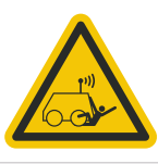
Run over by remote operator controlled machine
