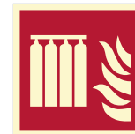
Fixed fire extinguisher battery
