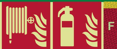
Low Location Lighting Systems shall include all necessary symbols for the escape route and fire-fighting equipment in addition to the IMO signs at eye level, according to ISO 15370 and SOLAS regulations. Our LLL mini symbols can be placed in staircases onto our Stair-Line LLL. The LLL mini symbols shall be the minimum height of 50mm according to the ISO 15370 standard.
