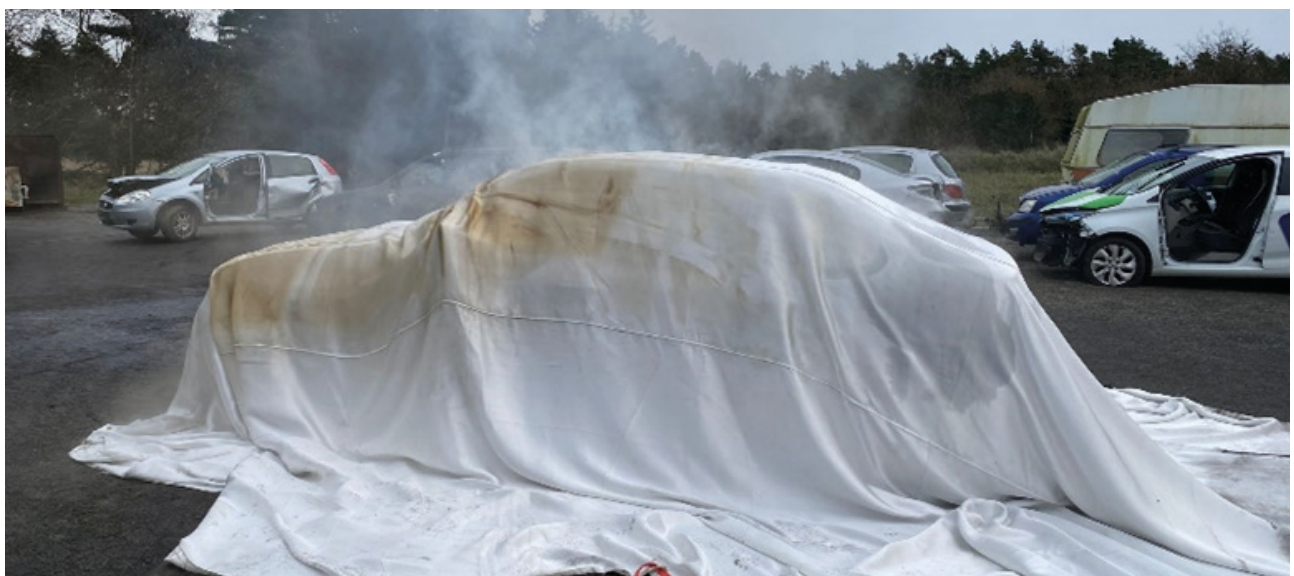
Blanket could stand temperature without any defects except discoloring due smoke
